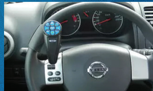
StickSteer Secondary Controller Steering knob that controls eleven secondary functions with thumb
