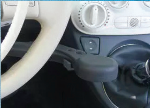
COLUMN MOUNT 907 Series Brake available for right or left side
