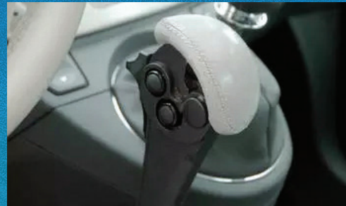
907 Brake Lever series Mount right or left on the column or floor mount
