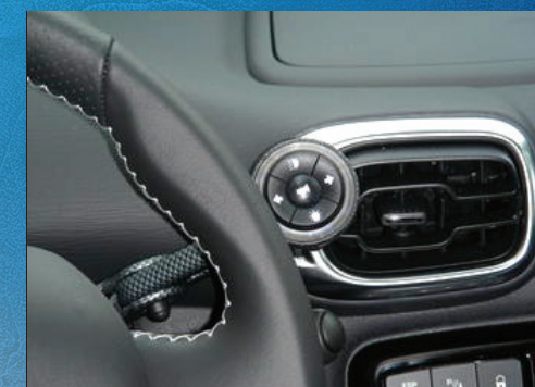
898 5 FUNCTION controller can be placed in handle
