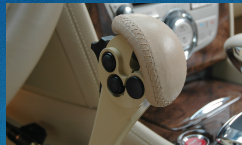
GT2 Accelerator/Brake Floor Mount Trigger or Rock Accelerator and push for brake
