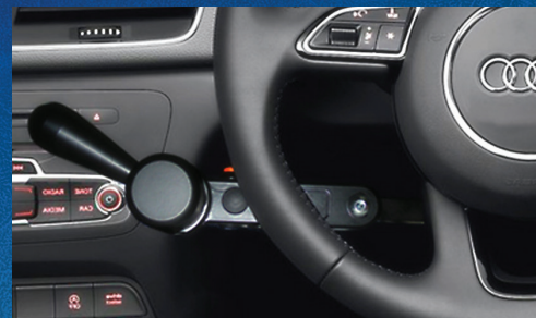
Modena Push Right Angle Accelerator/Brake Column mount left or special order right
