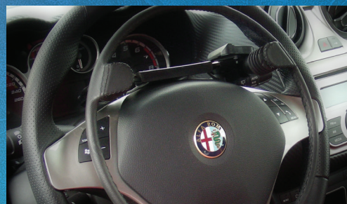
Over-Ring Accelerator Pairs with a 907 series brake lever
