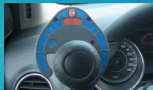
1094FV Secondary Controller Steering knob that controls eleven secondary functions with fingertips
