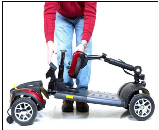
Figure 20. Connecting Frame and Drivetrain
