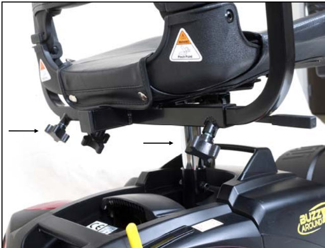
Figure 6. Armrest Width Adjustment
