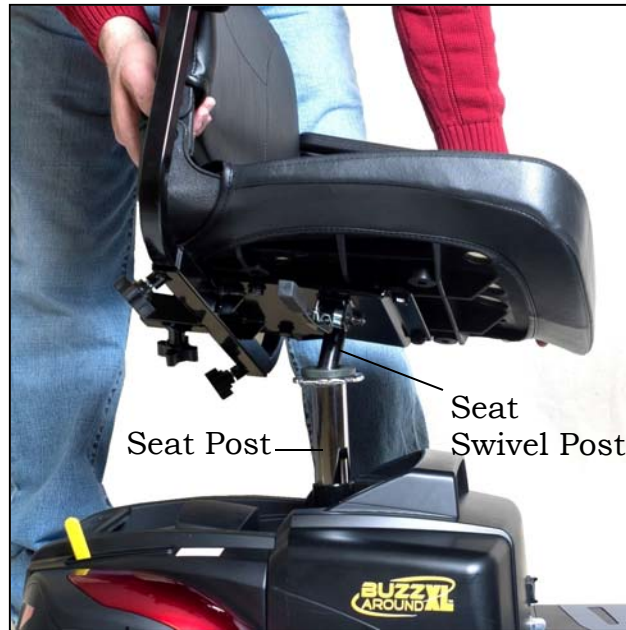
Figure 23. Installing the Seat
