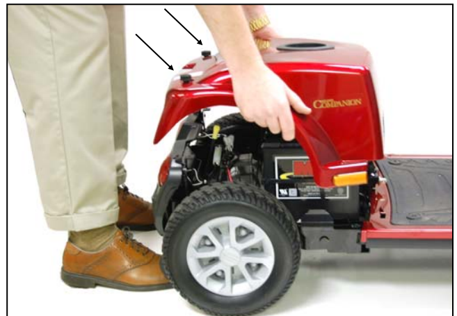
FIGURE 16. REMOVING THE REAR SHROUD
