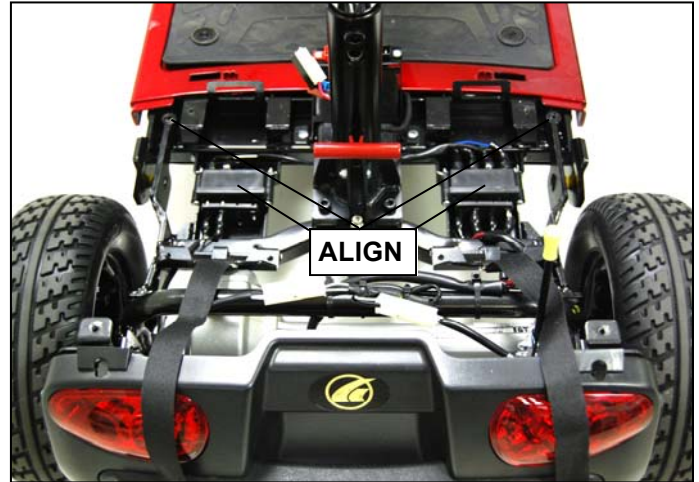
FIGURE 21. CORRECT FRAME ALIGNMENT
