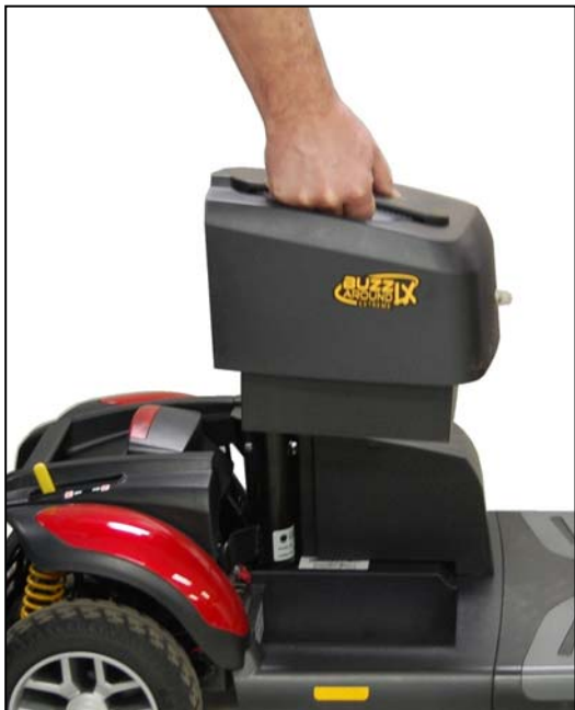
Figure 23. Battery Pack Installation
