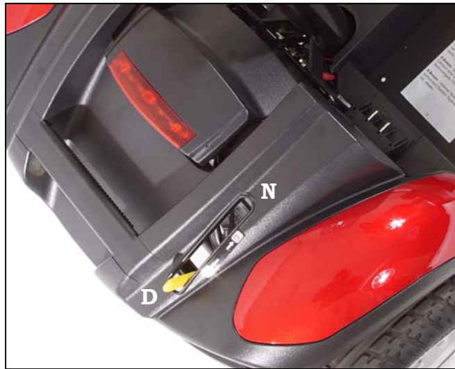
Figure 13: Freewheel Lever (Drive Position)
