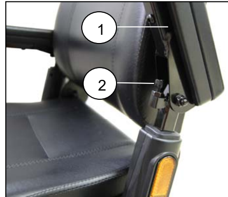
Figure 9. Armrest Angle Adjustment
