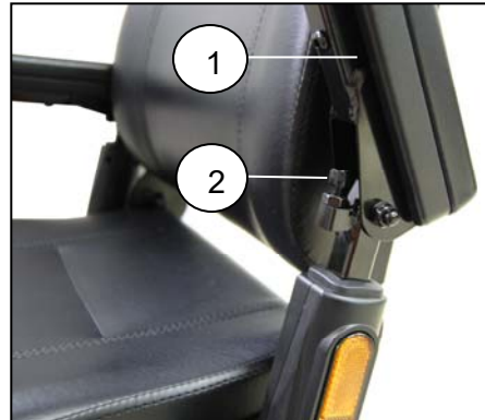
Figure 9. Armrest Angle Adjustment
