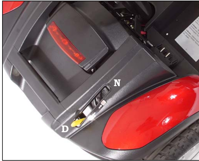
Figure 13: Freewheel Lever (Drive Position)
