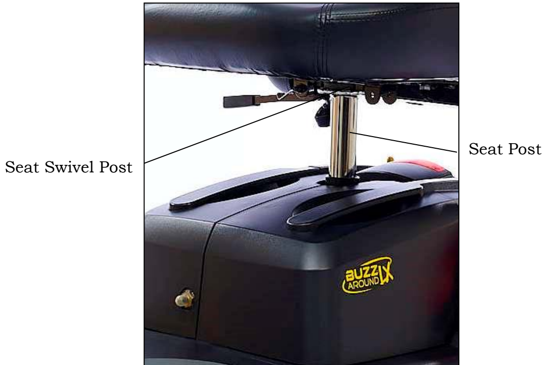
Figure 25. Installing the Seat
