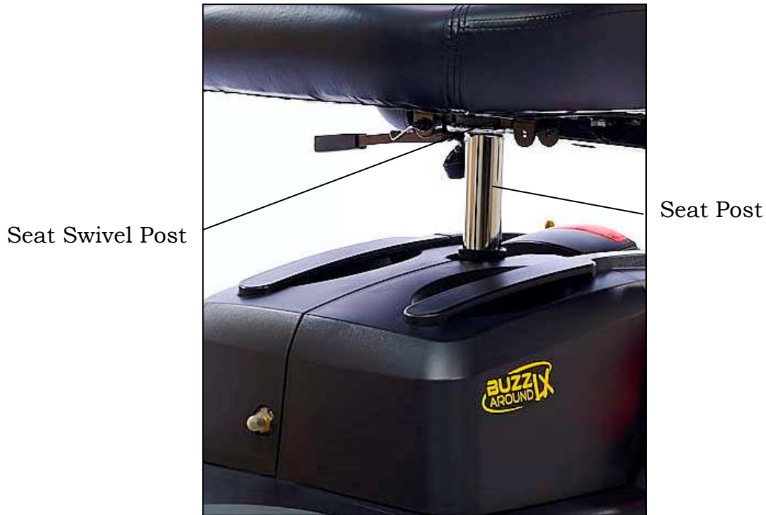
Figure 25. Installing the Seat
