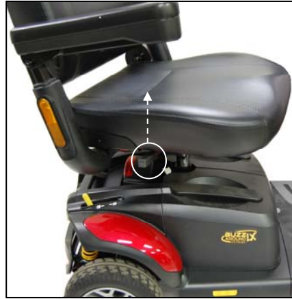
Figure 10: Seat Rotation Adjustment
