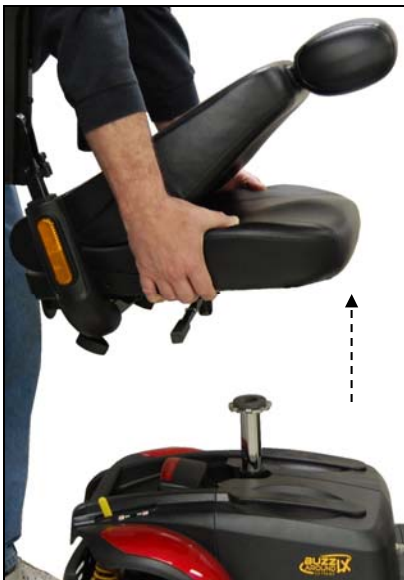
Figure 16. Removing the Seat
