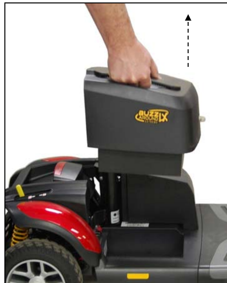
Figure 17. Removing the Battery Pack
