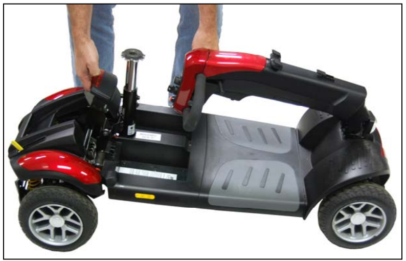
Figure 22. Connecting Frame and Drivetrain
