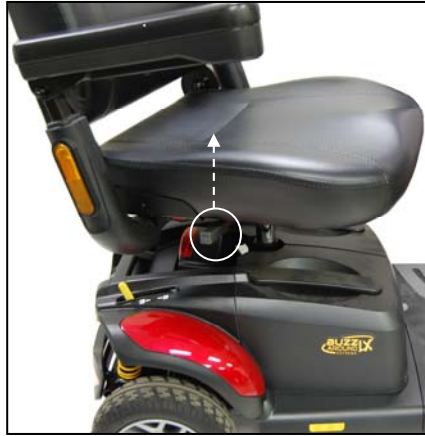
Figure 10: Seat Rotation Adjustment
