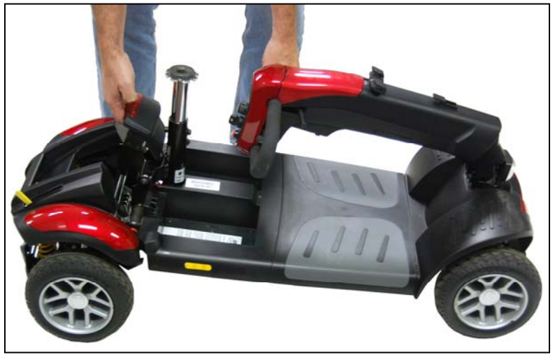
Figure 22. Connecting Frame and Drivetrain
