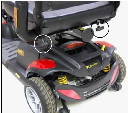
Figure 8. Armrest Width Adjustment
