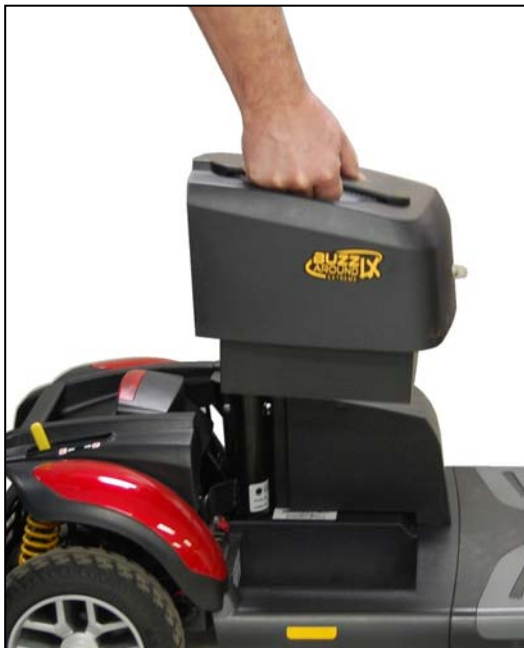
Figure 23. Battery Pack Installation
